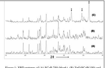
Figure 1: XRD patterns of (A) SCaP-750 (blank), (B) ZnO/SCaP(150) and (C) ZnO/SCaP(400)
